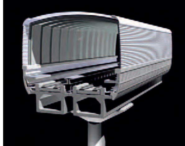
12. Design for full noise enclosure at crossings.
